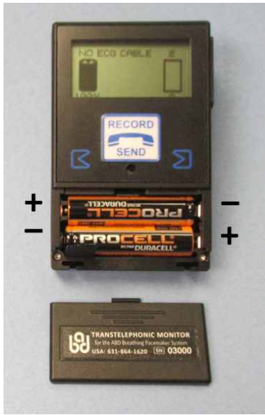
Figure 3. Battery compartment with door removed
