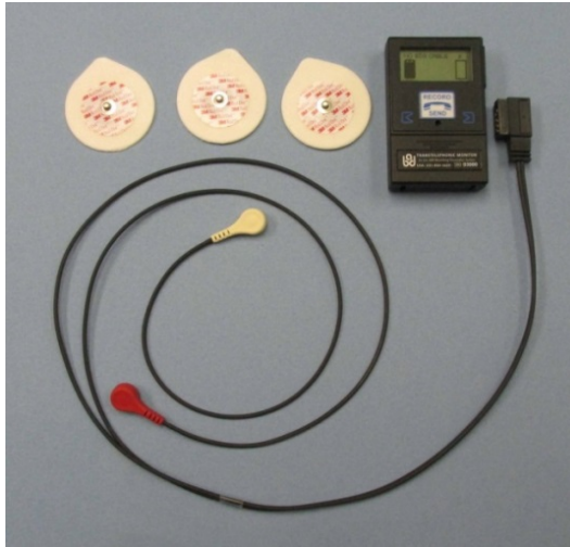
Figure 2. The TTM, cable and skin electrodes
